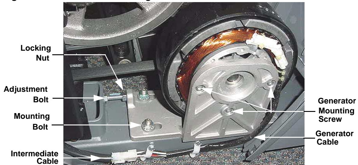
Diagram 7.7 - Generator Mounting
